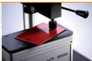
Determining the mechanical characteristics of lacquer coatings
