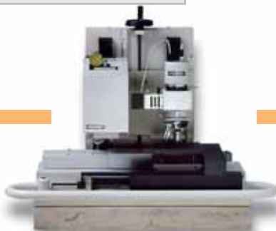
1999 FISCHERSCOPE® H100 C: Newly designed, with improved distance measurement, higher load resolution, integration of XY-control, new software
